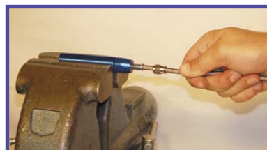
STEP 2 Flare braid using a twisting motion.
